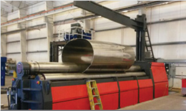
AHS 7700 x 9/12 CNC Four Rolls Hydraulic Plate Bending Machine / CNC Dört Valsli Hidrolik Silindir Bükme Makinesi
