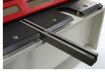
Çetveli, stoperli ve T-kanallı ön destek kolları T-slotted front support arms with scale and flip-stop
