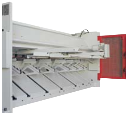
Pnömatik sac destek sistemi Pneumatic sheet support system
