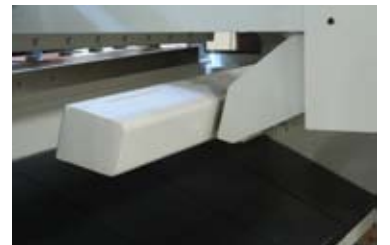
Kalkmalı tip arka dayama sistemi Swing-up backgauge system
