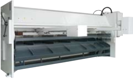
Universal pnömatrik sac destek sistemi Universal pneumatic sheet support system
